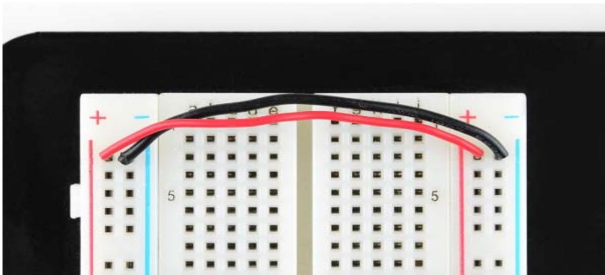
Two jumper wires used to connect the power rails on both sides.
