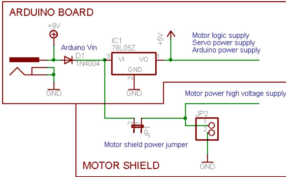
If you would like to have a **single DC power supply for the Arduino and motors**, simply plug it into the DC jack on the Arduino or the 2-pin PWR\_EXT block on the shield. Place the power jumper on the motor shield.
